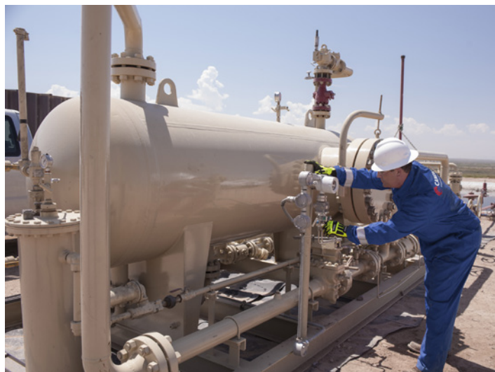
Low- and high-working-pressure vessels are used to separate oil, water, gas, and sometimes solids (sand) into individual streams for more accurate measurement and discharge control.
